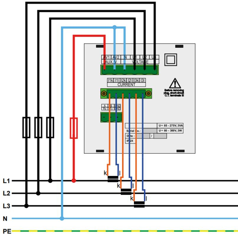
Figure 1: Multifunctional Measuring Device 3700X typical installation TN network, direct star connection ("3Y")
