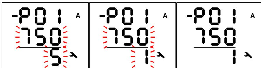
The target value for the current transformer is now set and the editing mode can be ended by (briefly) pressing **P**. The value is then stored in the device memory and no longer flashes.
