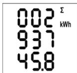
Each value uses three display lines, 8 digits before the decimal point and one after. Example on the left,  $\Sigma EP+ = 293745.8 \text{ kWh}$ .
