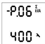
The parameters are arranged in groups, numbered from 00 upwards. The number of the group is shown in the first line in the format - *P.n n* (preceded by a dash). You can move through the parameter groups with the keys **▲** and **▼**.
