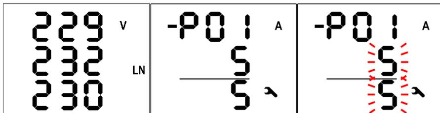
Now you can change the values. The first one is increased by pressing **▲**, and if you keep the key pressed, the value increases faster. For fine adjustment, press **▲** and **▼**.
