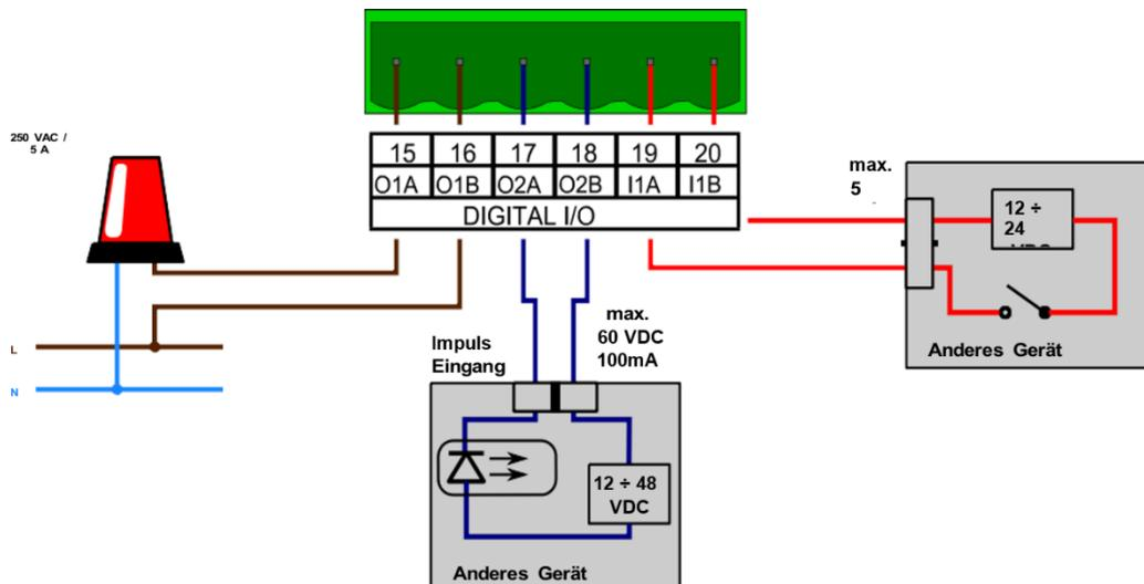
Figure 2: Connection example of the digital inputs/outputs. Output 1 in this example is a relay output (not standard)
