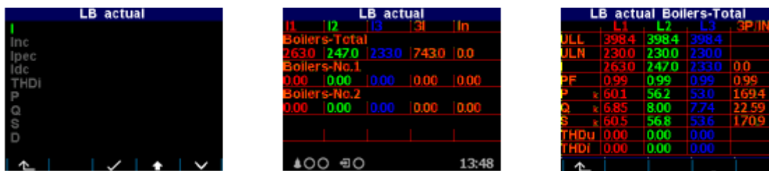
Figure 50: Actual values of the Local Bus modules on the display
