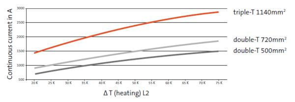
For the type verification corresponding to IEC/EN 61439-1, the maximum heating of the busbars must be taken into account.
